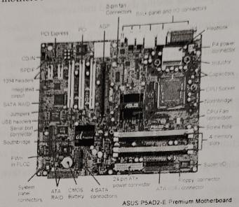
It is a printed circuit board that is the foundation of a computer, located at the bottom of the computer case. It allocates power to the CPU, RAM, and all other computer hardware components. Most importantly, the motherboard allows hardware components to communicate with one another.
